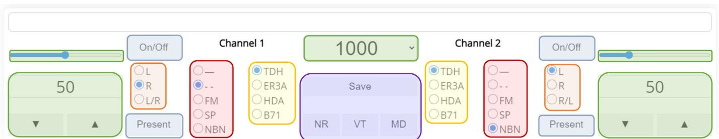
Figure 1. Virtual audiometer buttons colored by group. Red – sound selection, Orange – ear selection, Yellow – transducer selection, Green – sound properties, Blue – sound presentation, and Purple – save.
